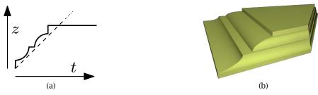
Fig. 4: (a) The height function used for obtaining the surfaces shown in Fig. 3(f) and 3(l). The standard height function which results in the roofs of Fig. 3(a) and 3(g) is shown by a dashed line. (b) Mitered chamfers based on a multiplicatively weighted straight skeleton also using the height function from (a).
