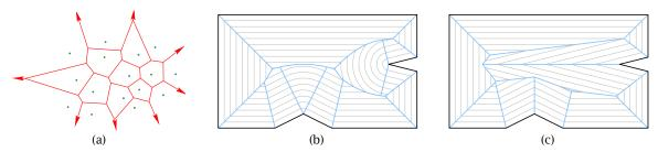
Fig. 1: (a) The Voronoi diagram (red) of 16 point sites (green). (b) The Voronoi-diagram (blue) of an input polygon P (black) with wavefronts (gray) at different times during the propagation process. (c) The straight skeleton (blue) of the same polygon.
